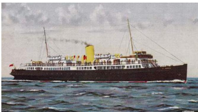
**TS *St Seiriol***: built by Fairfields in 1931; steam turbine; 1,586 gross tons; length 269 feet; speed 18½ knots; capacity 1,556 passengers. She was built as a smaller second ship to assist *St Tudno* and operate Isle of Man excursions. She was broken up in Belgium in 1963. (A Perrott)
